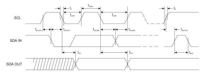
Figure 4-2. Write Cycle Timing: SCL:
