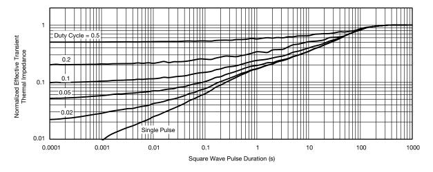
Normalized Thermal Transient Impedance, Junction-to-Ambient
