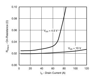
On-Resistance vs. Drain Current
