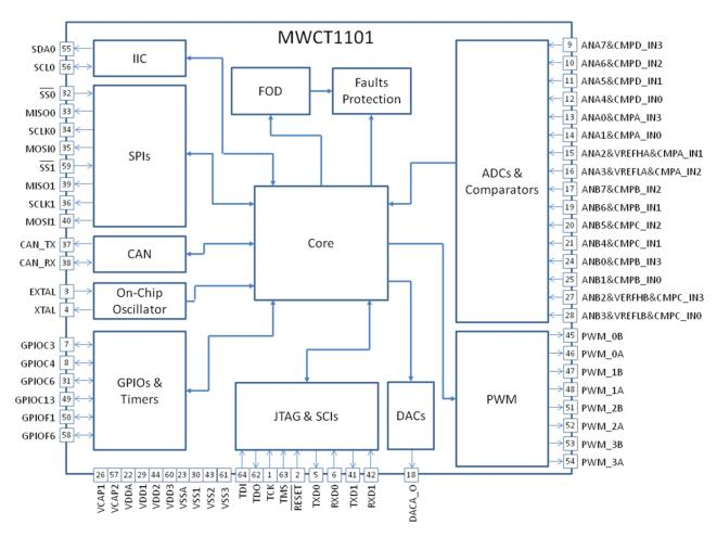
Figure 3. MWCT1101CLH Function Block Diagram
