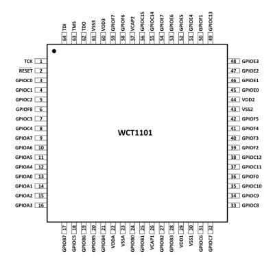
Figure 4. MWCT1101CLH Pinout Diagram
